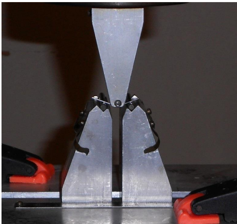
Figure 3. Three-point bending test in progress.
